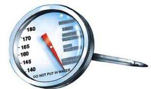
The bimetal food thermometer can accurately measure the temperature of relatively thick foods (such as beef roasts) or deep foods (foods in a stockpot). Because the temperature-sensing coil on the stem is between 2 to 2 1/2 inches long and the
