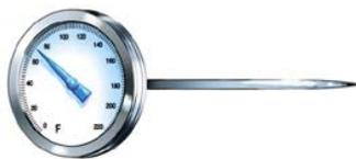
For accurate temperature measurement, the probe of the bimetallic-coil thermometer must be inserted the full length of the sensing area (usually 2 to 3 inches). If measuring the temperature of a thin food, such as a hamburger patty or boneless chicken breast, the probe should be inserted through the side of the food so that the entire sensing area is positioned through the center of the food. Some models can be calibrated. Check the manufacturer's instructions.
